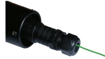
The connector can now be removed from the WindSonic.
