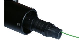
Now screw the cable-clamping nut into place.
