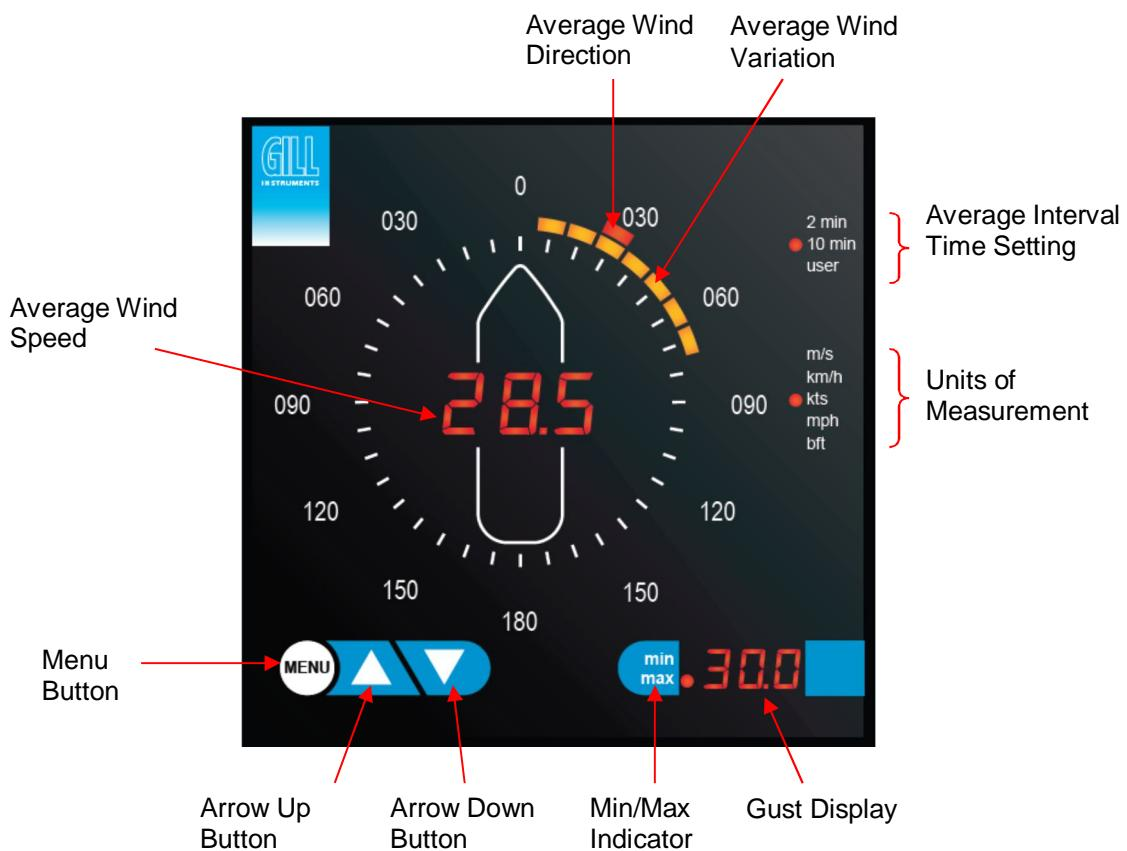
On the front panel of the display there are three push buttons, “MENU” “▲” and “▼”. An explanation of front panel button functions is as follows:-
