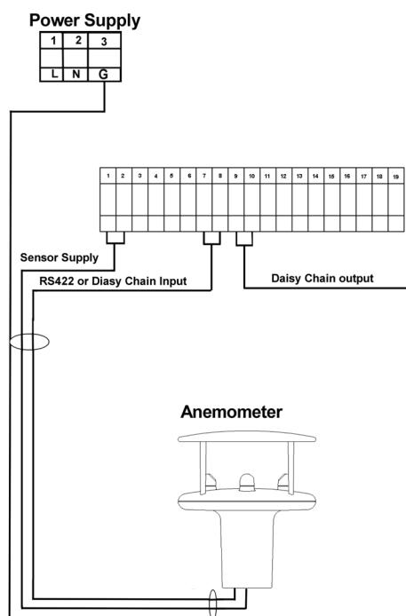
When both the anemometer and display are powered on wind speed data should be read on the 3 digit speed display and direction data indicated by the outer circles of LED's. The information update rate will be once per second.
