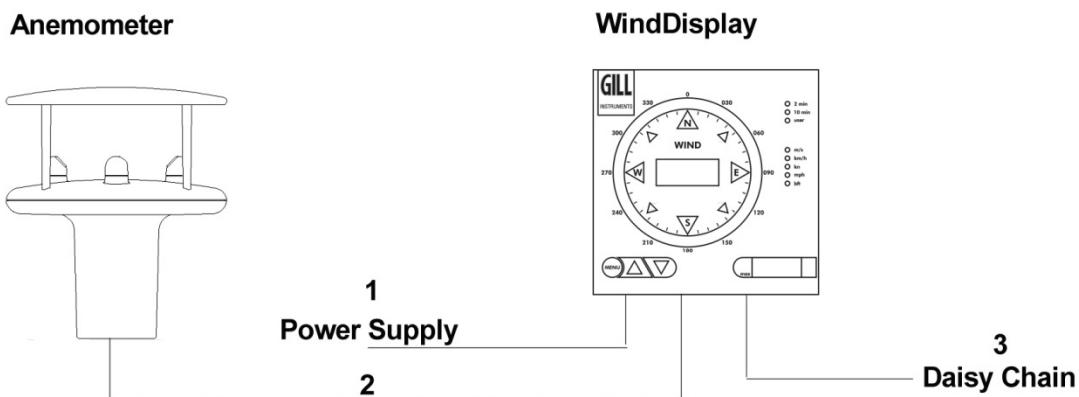
**1** = 3 core mains cable 1.00 mm<sup>2</sup> 10A rating
